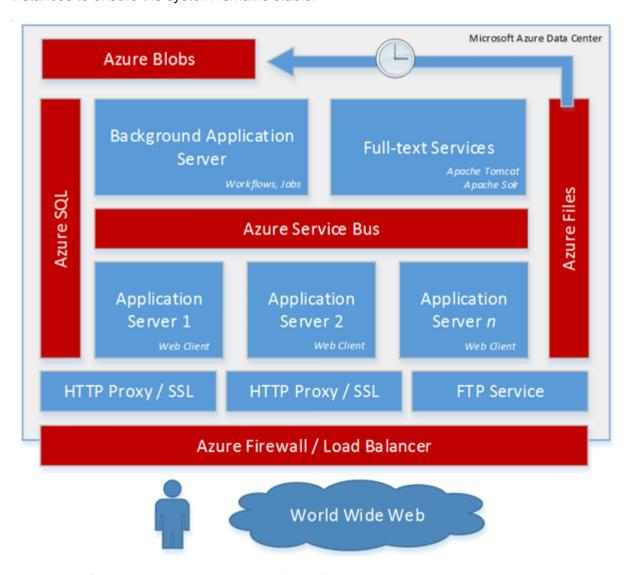
DocuWare Cloud builds on the Azure platform. The red components belong to the Azure platform, the blue components to the DocuWare Cloud.
